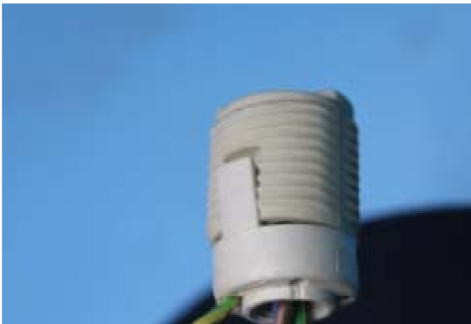
Photo 23 Alternative construction of G9 lampholder for all models
